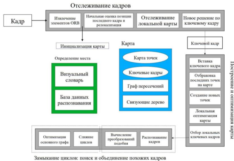
Рис. 2. Система ORB-SLAM ( https://courses.cs.washington.edu/courses/csep576/21au/resources/ORB-SLAM_A_Versatile_and_Accurate_Monocular_SLAM_System.pdf )
