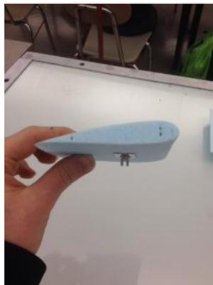
Image 5. Airfoil with the mounting tab
