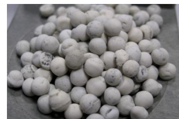
Fig. 5 Porcelain media diameter 5 mm
