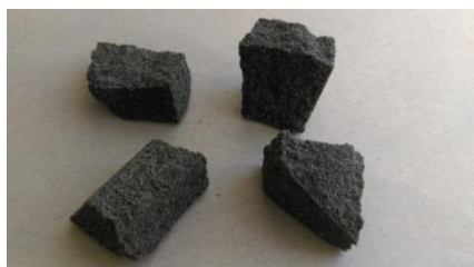
Fig. 3 Aggressive deburring media, rit 25
