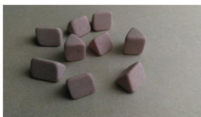
Fig. 4 Triangular prisms 15x15, grit 16
